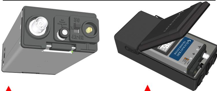
Top end panel includes BNC jack, ground screw, whip band switch, & whip mount. Battery can be accessed via the hinged back cover.
